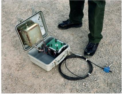
• Seismic Sensor, New Mexico.
